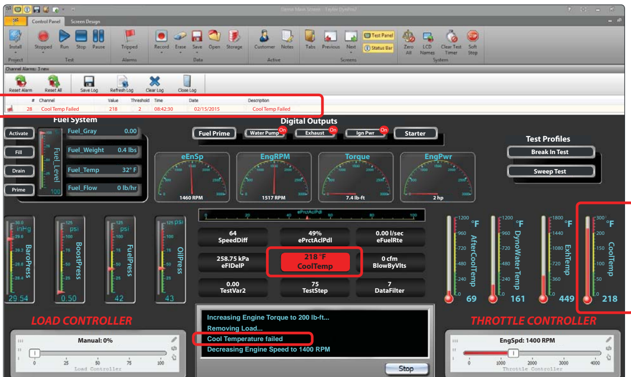
User screen with 4 channel alarm notification examples
