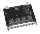
The Model 7003-8-TC Thermocouple Input Card is used in conjunction with the Model 7003-8-A-I Analog Input Card to perform signal conditioning and cold-junction compensation for thermocouple types J, K, T, E, N, R, S, and B.
