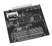
The Model 7003-8-A-I Analog Input Card performs the analog anti-alias filtering, analog-to-digital conversion and data storage for the System. The Model 7003-8-A-I is used in conjunction with a Sensor Input Card, which performs the sensor-specific analog conditioning.
