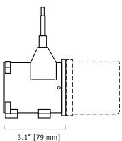
Our unique linear-to-rotational, industrial-grade string encoder module mates to virtually any encoder giving you a cost-effective linear position measurement solution that precisely fits your requirements. The PT8600 takes just minutes to install, fits easily into tight areas and does not require perfectly parallel alignment. To order, simply select the stroke range, the cable tension and the mounting style that matches your encoder.
